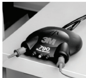
Figure 6: 3M™ Static Monitor 790 attached to equipment chassis
